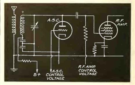
Automatic selectivity control as applied to the antenna stage of a receiver. The plate impedance of the triode varies the selectivity.
