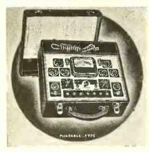
Tube analyzer with free point analysis—possibility of obsolescence eliminated—accommodates over 300 types. Line voltage checked on meter—instrument fused. Provides hot inter-electrode short and cathode leakage tests—each portion of multisection tubes checked separated. Tubes tested under load—condition indicated on direct reading scale. Avail-
