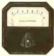
★ DS meter of D'Arsonval type with unusually long scale (4½ in.)—jewelled pivots. Semi-flush type mounting—bakelite case. Accuracy within 2 per ceni—made in all popular current and voltage ranges. Mounts through 2¾ in. diameter hole. Hoyt type 573—10 milliampere movement—list \$8.50. Burton-Rogers Co., 755 Boylston St., Boston, Mass.—Radio Today
