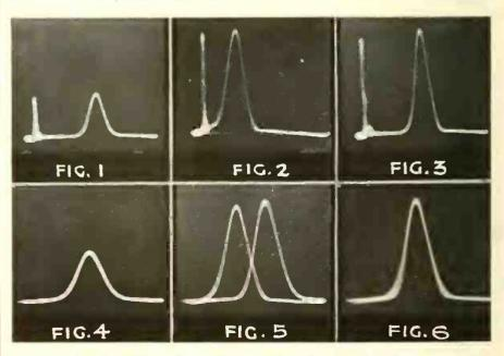
The cathode-ray oscillograph provides a means of seeing the alignment of the receiver. The oscillograms shown illustrate alignment of the oscillator at 600 kc.
