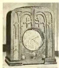
★ Line of all-wave receivers using 8-inch tuning dial with phantom illumination for ease of tuning and calibration-dual ratio vernier. Table and console models with six to ten tubes — combination of metal and
