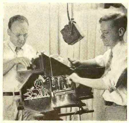
Studio engineers using the iconoscope television camera for direct pick-up of actual scenes. The image is focussed on a photo-electric mosaic scanned by a cathode-ray beam electromagnetically controlled.
